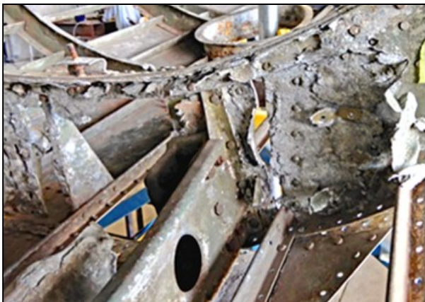
Left: a badly corroded section of the DC-2
