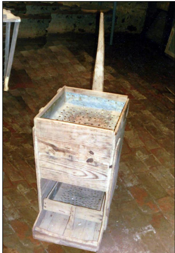
Cradle displayed at Jindera Pioneer Museum used to separate gold from surrounding material.
