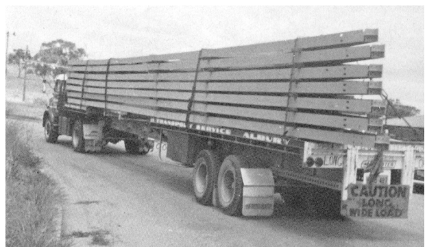
Extendable trailer transporting long roof trusses for AB & MA Chick c.1964
