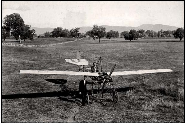
On Tuesday the experiment was repeated in the presence of a Banner representative and the machine took to the air gracefully. The trial, however, was interrupted by a mechanical de-fect, but the test demonstrated the capacity of the monoplane to take to the air after a ground run of about 200 yards. The inventors, who deserve to be rewarded for their patience and industry, intend exhibiting their machine at the coming Albury Show.
